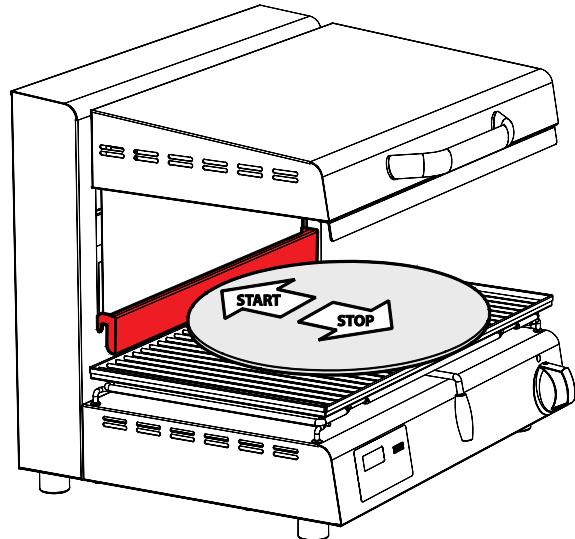
If there is a power failure during cooking, when power returns the remaining cooking time will flash on the display. By pressing "START" the appliance will start again from this point.
